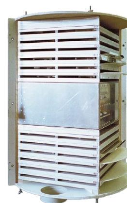
Sieve stack with encapsulated driving unit
