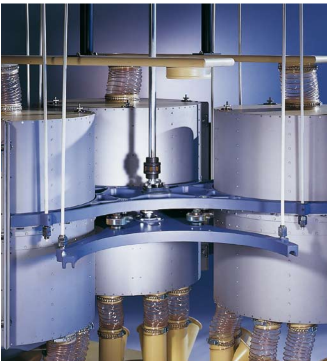
The cross yoke drive system, one sieve stack removed.
